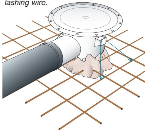
(Alt.2) Recess: when the waste pipe is embedded, a recess is made of e.g. rockwool in the form, with the size 300 x 300 mm.
