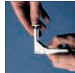
A gentle pressure on the middle of the arm releases the knife holder and the blade
