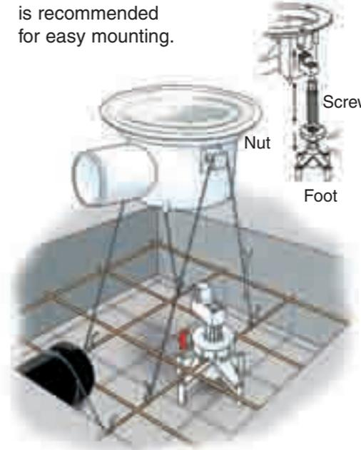
(1) Nail the foot and turn the nuts on both feet up to the right level. The height can be adjusted 60 mm. With an extra sleeve 110 mm.
