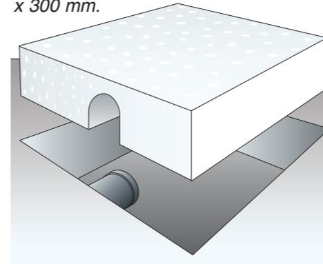
When the concrete has burnt, the floor gully is placed in the recess/hole and is connected to the outlet pipe.
