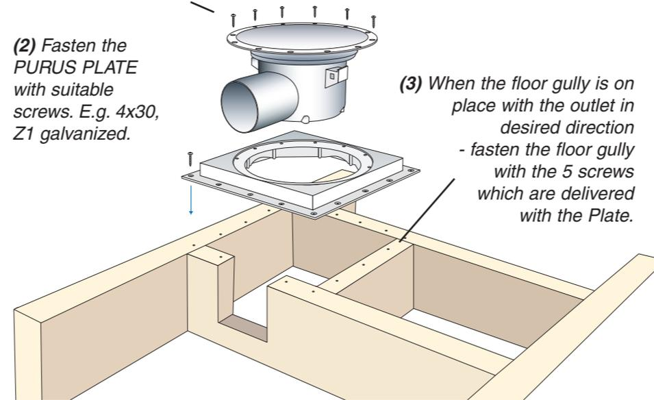
(3) When the floor gully is on place with the outlet in desired direction - fasten the floor gully with the 5 screws which are delivered with the Plate.
