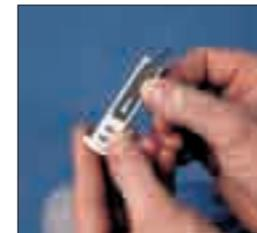
To change the blade, the holder is pulled up. Blade: Stanley 5903.
